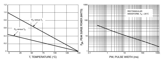
Figure 3. Steady State Power Derating
