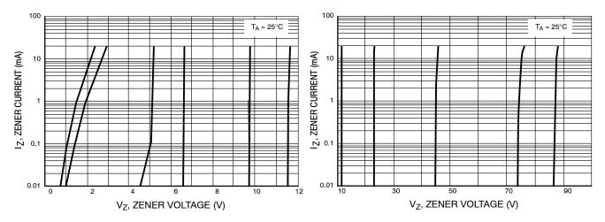
Figure 9. Zener Voltage versus Zener Current (V<sub>Z</sub> Up to 12 V)
