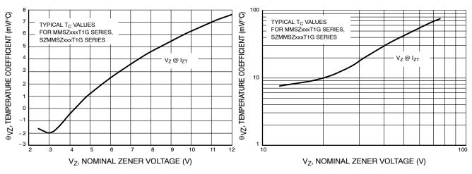
Figure 1. Temperature Coefficients (Temperature Range –55°C to +150°C)
