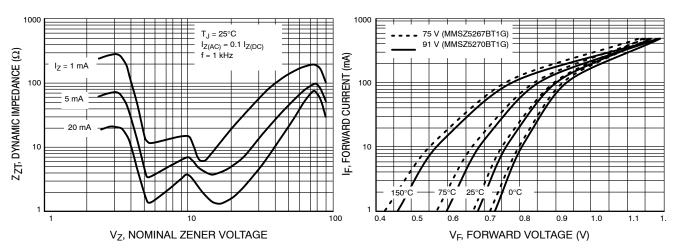
Figure 5. Effect of Zener Voltage on Zener Impedance
