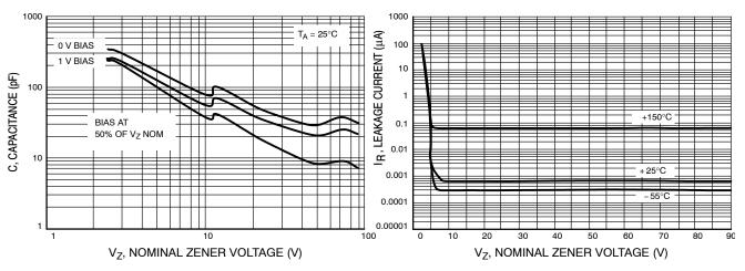
Figure 7. Typical Capacitance
